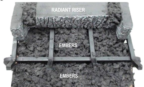
STEP 4: Stuff the embers into the notches of the Radiant Riser and cover all visible burner media as shown in figure 4. Now install the Radiant Heat series logs according to the log diagram sheet included with you log set.
