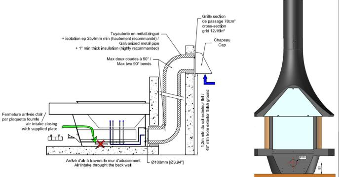
Caution: the Outdoor Combustion Air intake must not come from an attic, garage, carport, basement, the chimney's enclosure or be less than 3m (10') from a gas meter, a fuel/propane tank or any other device that may emit fumes or gases, such as the exhaust of a motor vehicle.
