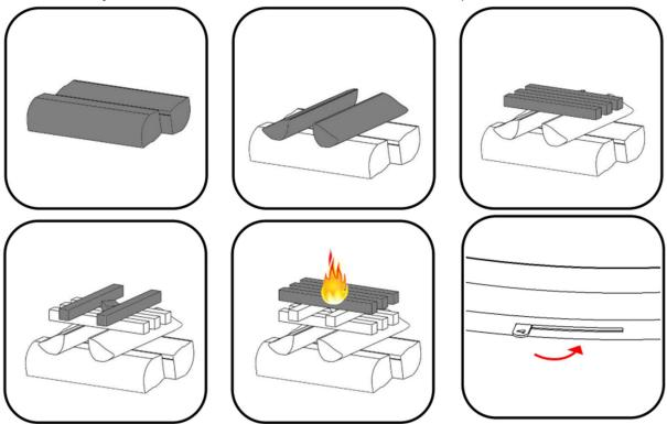
REMINDER: The ignition of the appliance must be carried out using this ignition method (reverse ignition).
