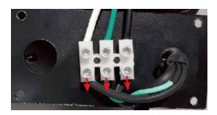
2. Attach the wiring to the junction block. Please make sure the live wire goes into the "L", the neutral wire into "N" and the ground wire into "G".
