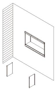
7. Insert the front glass panel back in place after the media installation has been completed.
