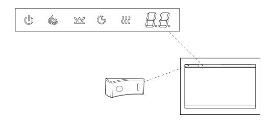
Touch the control panel once to "wakes up" the controls. This will cause the controls to light up. At this time, you can press the power button to turn on fireplace
