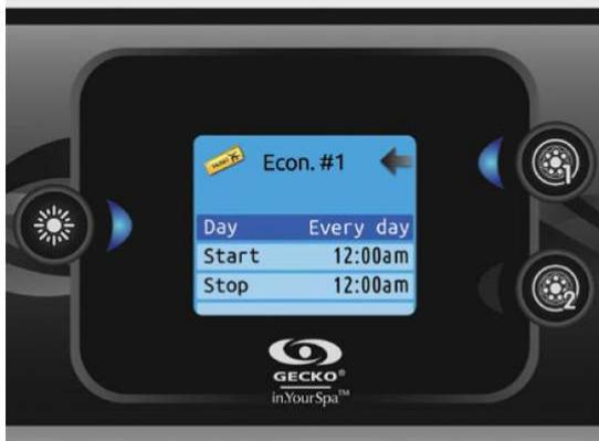
The filtration schedule shown on the screen will apply to the main filtration pump, most likely pump 1.
