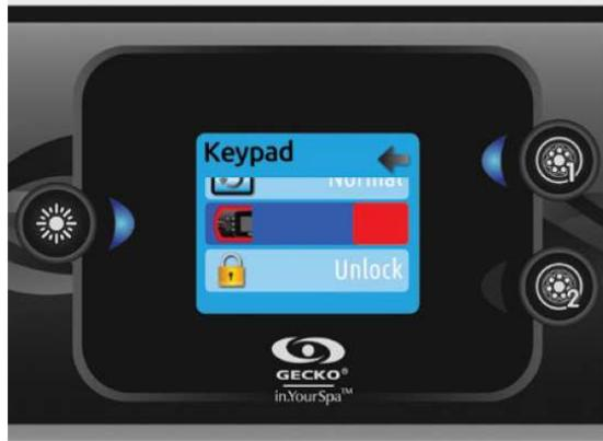
With the in.k500 equipped with a selectable rim light color modul: If the "RGB backlight" option is enabled in the spa configuration an option will appear to allow selection of the keypad rim light color.
