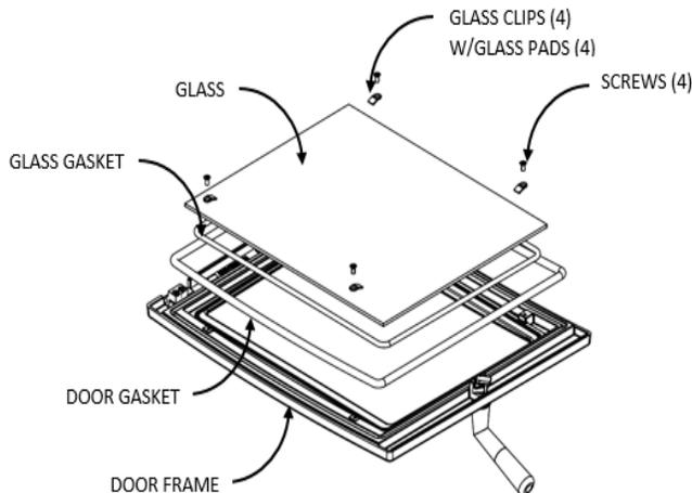
Gasket = Cordon d'Étanchéité (Joints) Door = Porte
